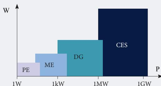
Legend: PE – portable energy; ME – mobile energy; DG – distributed generation; CES – centralized energy supply
